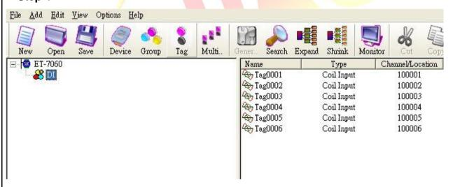
You could communicate with DI of ET-7060 now. You could also add other tags as the same way just notice the difference of address and Prototype.
